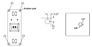
Fasten screws into a firm wall or wall support as shown in the figure, and hang the holes of the mounting bracket on the protruding screws.
